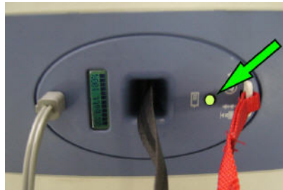
Figure 4D - Hoist ON indicator
