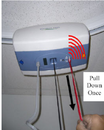
Figure 10A - Pull down on the RED CORD once to stop the hoist. The unit will beep once and all power to the hoist will be turned off.
