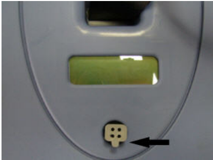
Figure 13A - Grey rubber grommet located on underside of hoist. Rubber airline is not connected. Note grey rib on grommet.
